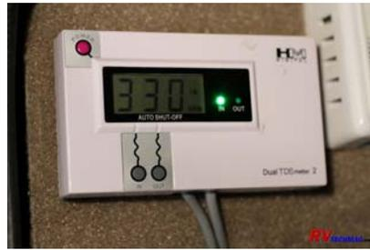
A TDS meter was added to check the condition of the deionizer media
