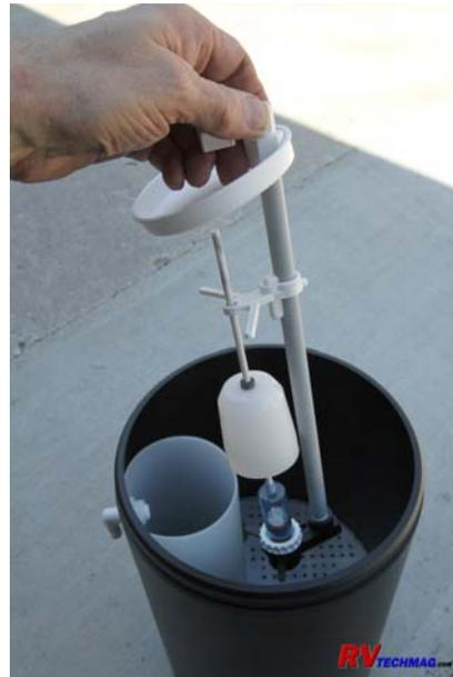
The rubber band needs to be removed from the float prior to use
