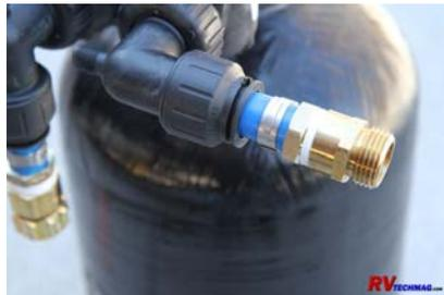
Pex to garden hose thread adaptors were made to adapt the softener and deionizer to flexible hoses
