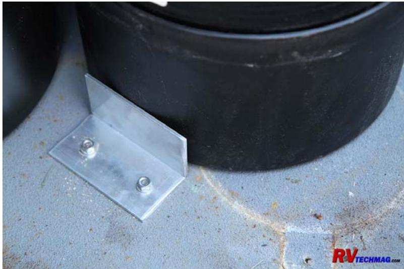
Aluminum brackets were made to keep the equipment from moving around in the tray
