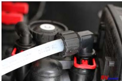
Polyvinyl tubing was run from the softener to the gray water tank to accommodate the water flow when backwashing the system
