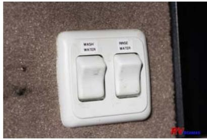
A pair of rocker switches selects the water supply to the deionizer
