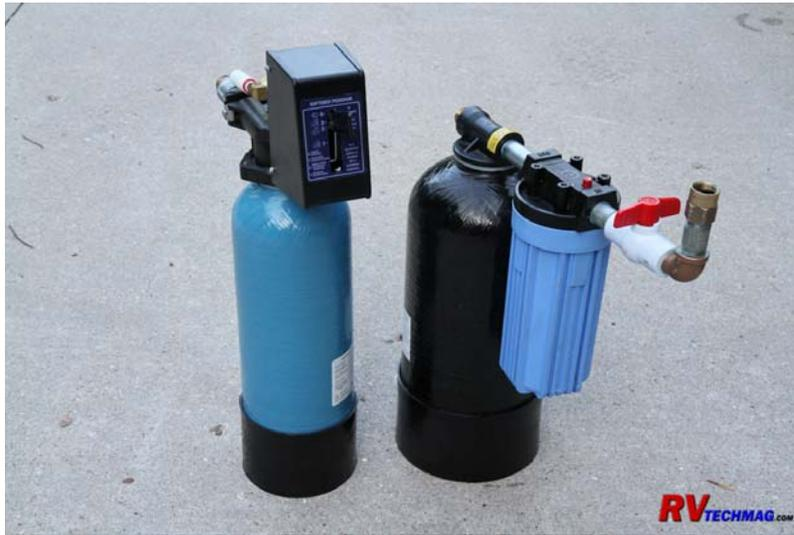
My original system consisted of a water softener with pre-filter as well as an iron filter
