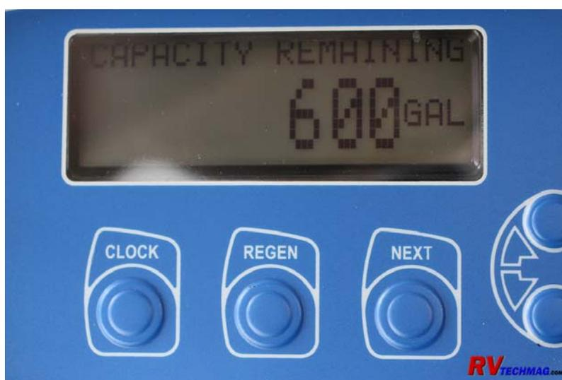
The water softener control features an easy to read LCD display
