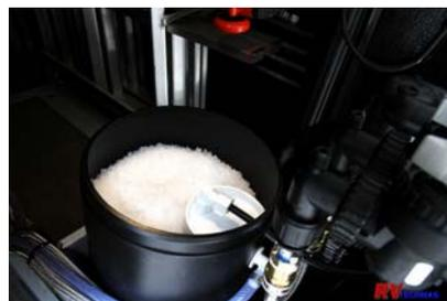
The overflow hose was attached to the brine tank and the tank was filled with solar salt
