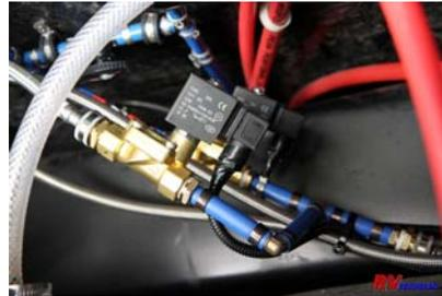
A pair of 12 volt solenoid valves controlled water to the deionizer
