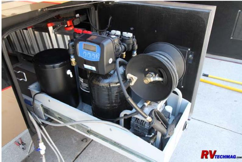
Hard water is found in many areas of the country. The hard water available at some RV parks can cause plenty of ill effects to your RV. These can range from soap scum that doesn't rinse off to calcium deposits on dishware to damage to your plumbing fixtures. To rectify this you need a water softener.
